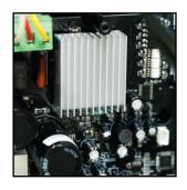
Built-in Heat Sink Improving the heat dissipation and provide a total cooling solution for even challenging thermal environments.
